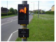
At toucan crossings, pedestrians and cyclists can cross together. Pedestrians or cyclists wishing to cross can press the button on the yellow box to stop the traffic. Detectors monitor the
